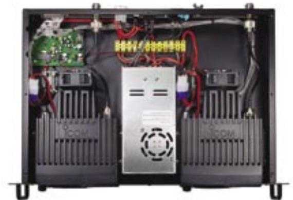
*Radios, controller, and power supply, all in one box. Dual forced-air fans keep the unit cool. 19" Rack mountable. Battery backup capable.*
